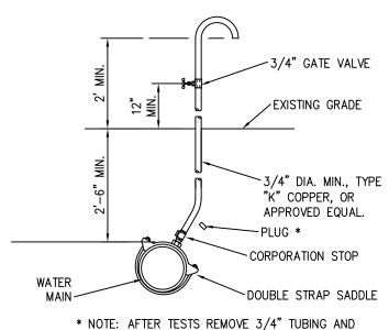
INSTALL PLUG ON CORPORATION STOP. TYPICAL BACTERIOLOGICAL SAMPLING (304) POINT AT INTERMEDIATE POINTS
