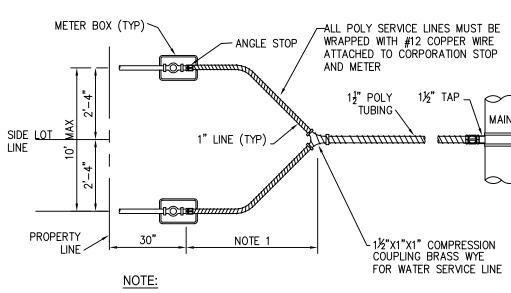
KEEP 11/2" WYE AS CLOSE AS POSSIBLE TO METER BOX. DOUBLE NEW SERVICE PLAN
