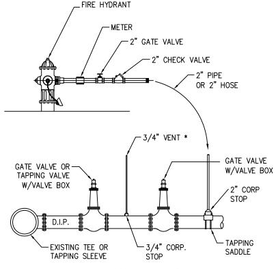
\* NOTE: AFTER TESTS REMOVE 3/4" TUBING AND 2" GALVANIZED PIPE AND INSTALL PLUGS ON CORPORATION STOPS.
