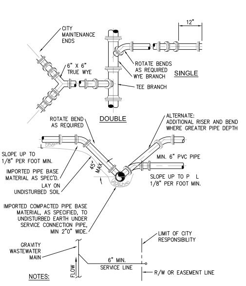
WASTEWATER MAIN WYE BRANCH TO MATCH MAIN PIPE MATERIAL. 2. NO 90° BENDS SHALL BE USED FOR WASTEWATER SERVICE AND
