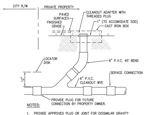
SEWER PIPE FOR SERVICE CONNECTION. . CLEAN-OUT ASSEMBLY SHALL BE INSTALLED BY PROPERTY OWNER.
